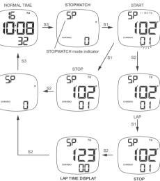
Press S2 to reset the stopwatch.
