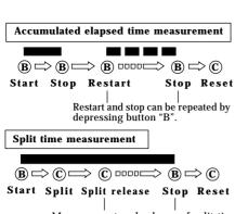
Measurement and release of split time can be repeated by depressing button "C".
