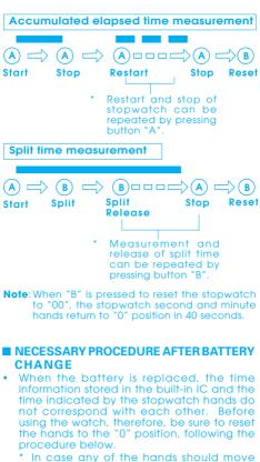
In case any of the hands should move improperly, follow the procedure below to adjust the hand movement.
