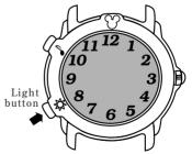
Note: When the electroluminescent light begins to lose its luminance, this is an indication that the battery is depleted. In this case, we recommend that you change the battery with a new one. LUMIBRITE WATCH (dial, hands, buttons, case, bezel, strap, etc.)
