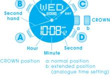
The caliber NX11 and NX14 have the different designs of digital displays, but their usages are the same. The following sections of this manual will provide explanation by using the caliber NX11 as an example.
